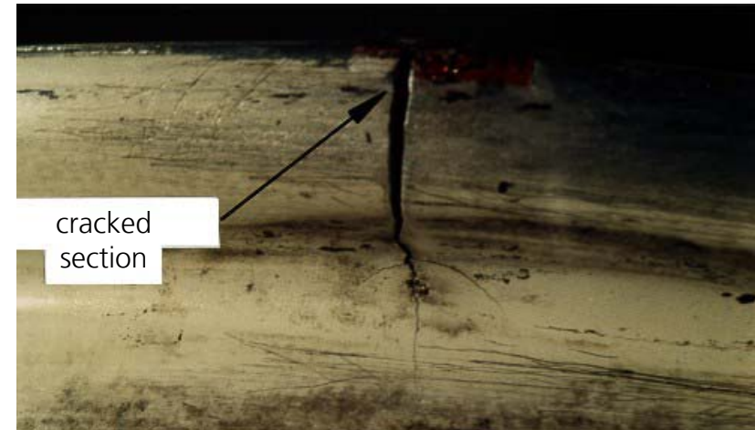
Fatigue Crack after validation test
