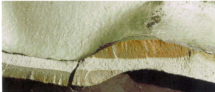
Fracture after \approx 200\,000 \text{ km} Service usage
