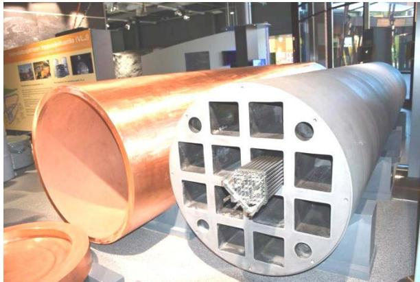
Underground Storage Canister Model for highly radioactive nuclear waste
