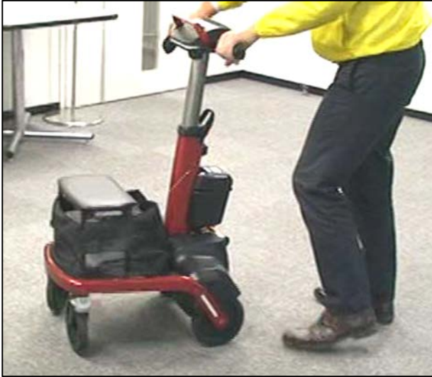
Picture 3.4: Robot Assist Walker RT.1 in operation.
