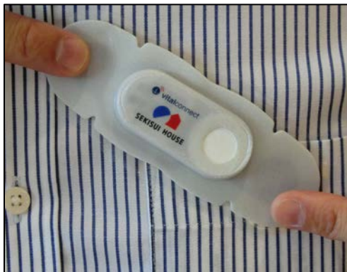
Picture 3.6: Patch-type sensor attached to the skin at the chest.
