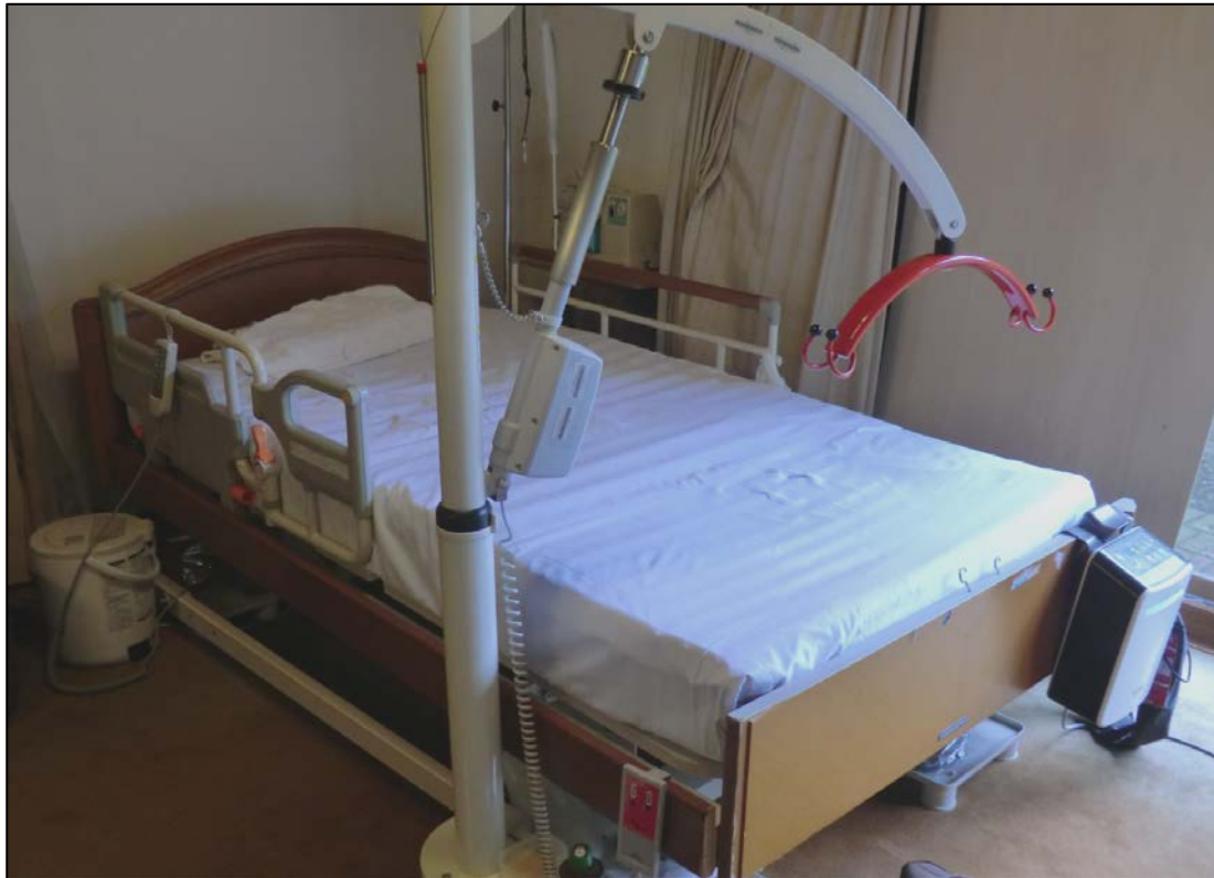
Picture 3.1: Transfer assistance lift Tsurube B-set attached to a hospital-type bed.
